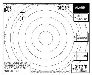
(1) Drag cursor to top (or bottom) corner for guard zone and press the A:SET GUARD1 or C:SET GUARD2 soft key. The soft keys disappear and the instruction box appears at left-hand cursor.
